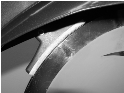
Correct pad gap
